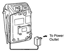
Tuck the telephone line cord inside the wall mounting adaptor, then push it in the direction of the arrow.
